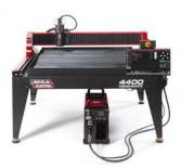
**Plasma Cutter -** Consisting of production components built into small machine footprint, allowing real world manufacturing tools to teach CNC operations, grasping CAD and CAM design.
